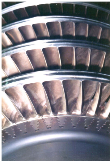
(a) Three dimensional flows designed Integral shroud blade (ISB)
